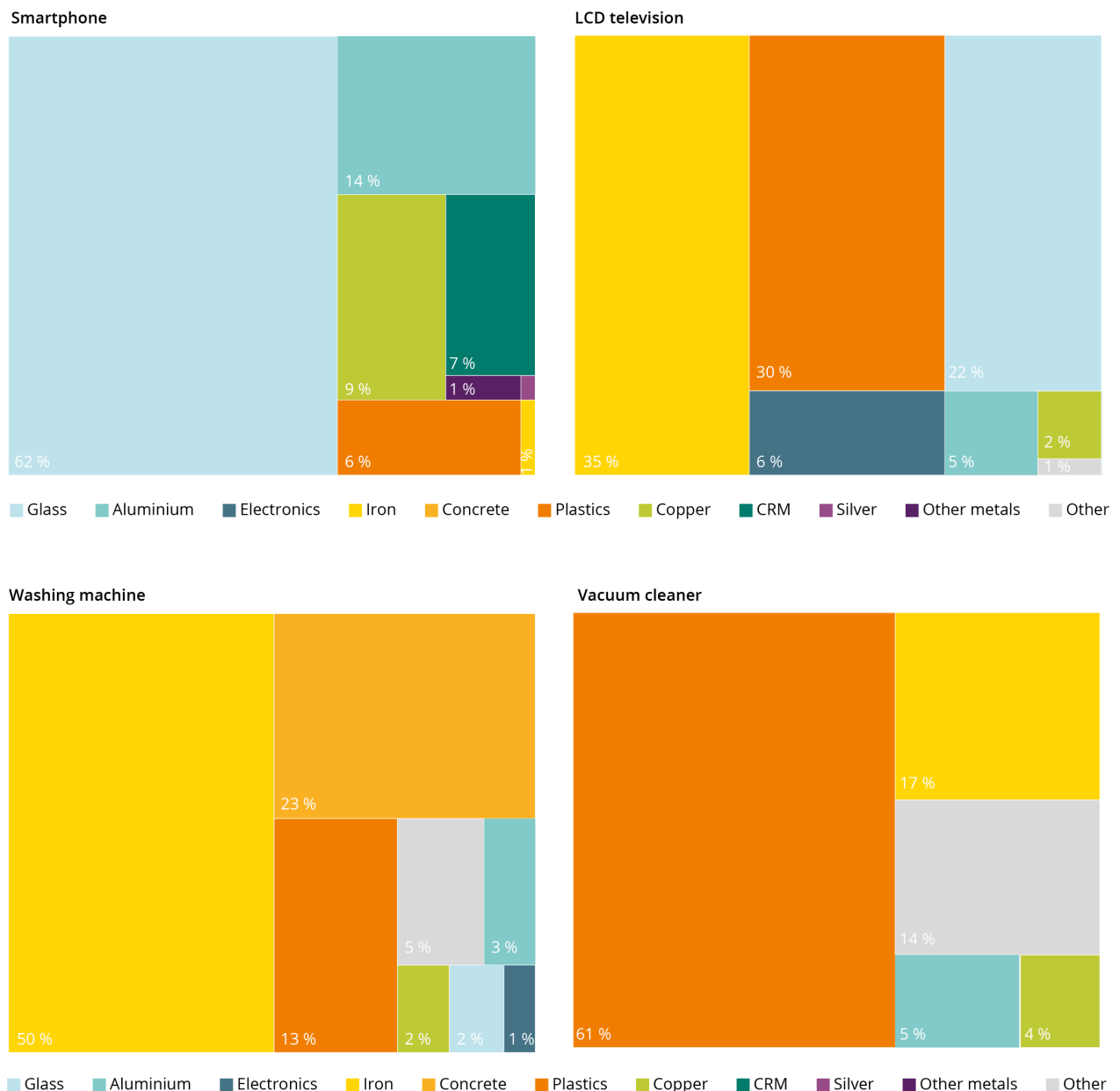
Figure 2.12 Average composition of smartphones, liquid crystal display televisions, vacuum cleaners and washing machines, per cent by weight
